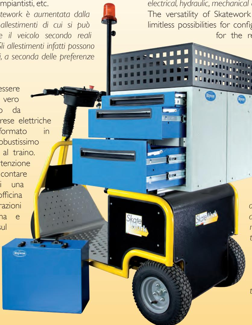
This is the ultimate Skatework configuration for the maintenance technician. The kit includes removable drawers and cases for power tools, internal and external compartments for fastener hardware and specialised compartments for carrying specific materials for a wide variety of maintenance jobs: such as electrical, hydraulic, mechanical and plant maintenance.
